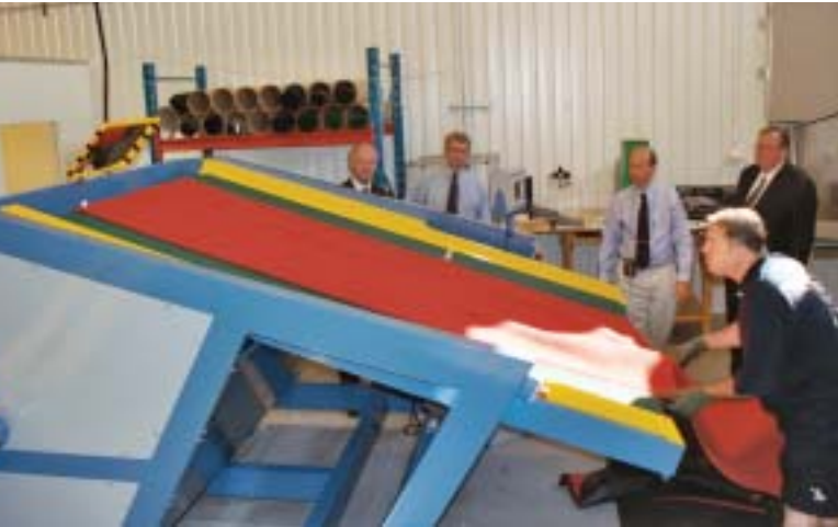
Brad Dorel loads a 5-meter mat using the height-adjustable conveyor.
